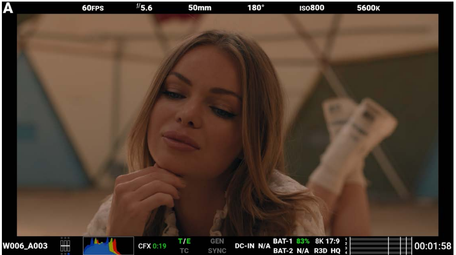
Figure: SDI monitor with SDI Advanced Overlay Mode enabled
